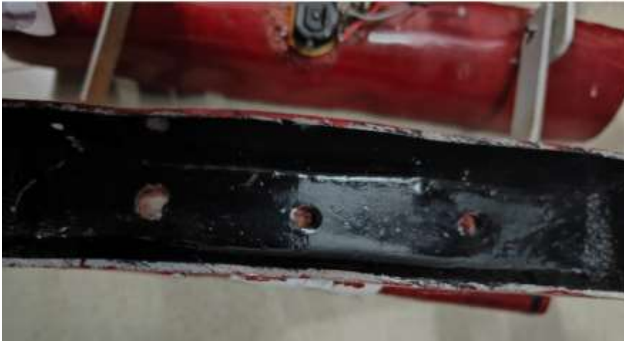
Figure.17. Seed Feeder holes are opened
