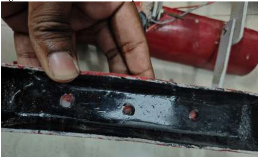
Figure.18. Seed Feeder holes are closed
