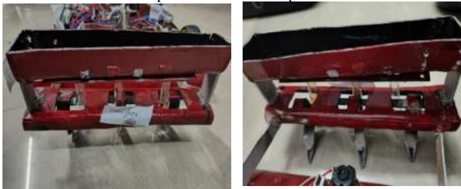
Figure.15.Mobile Application shows the Seed feeder ON The seed feeder holes are open and closed for a particular time interval.
